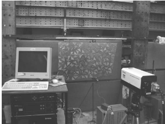
Fig. 18. Experimental set-up, showing logging PC, plate with attached damping and scanning laser vibrometer.
